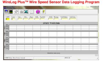
The WireLog Plus<sup>™</sup> Program is used with the SmartSensor and provides a simple MODBUS terminal to program and to download data from multiple SmartSensor<sup>™</sup> devices. The program uses the MODBUS<sup>™</sup> RTU protocol to establish communication with multiple SmartSensor devices. The interface to the Sensor is via a RS-485 duplex network.
